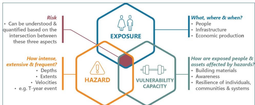
Figure 2-1 Framework for risk assessment, illustrating the relationship between hazard, exposure, vulnerability, and risk
