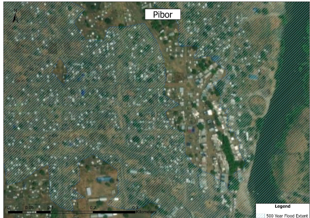
Figure 2-4 Example: satellite image representing land use/cover and buildings overlaid with selected simulated flood extent
