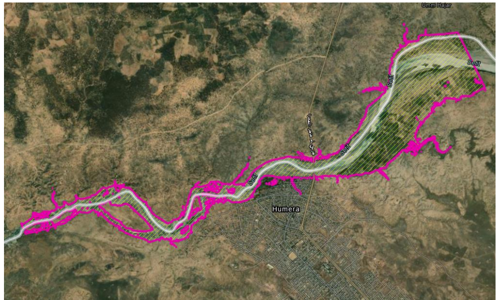
Figure 51 Flood extent for the 100-year flood event for at Humera.
