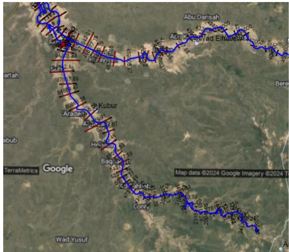
Figure 25 Angereb branch added to the model and secondary branch just downstream of the dam on the left side of Atbara.
