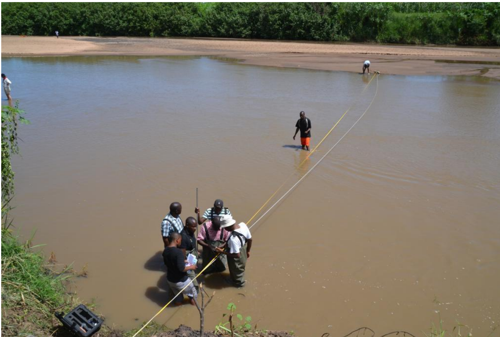
Figure B-3: A team of Hydrologist conducting low flow measurements at Mara mine
