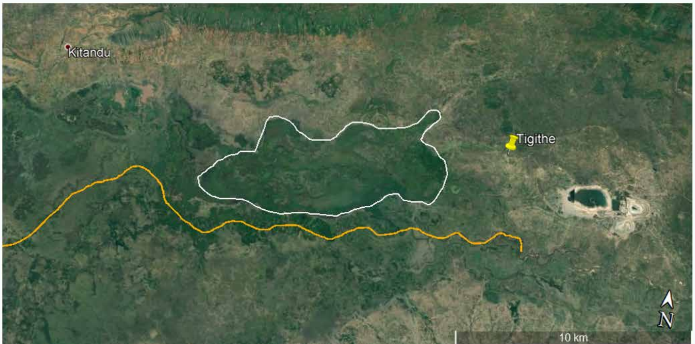
FIGURE 4 38: A GOOGLE EARTH IMAGE SHOWING THE BACK SWAMP (ENCIRCLED BY THE WHITE LINE) FORMED BY THE ALLUVIAL RIDGE/LEVEE (BROWN LINE) ALONG MARA RIVER. THE TIGITHE RIVER DRAINS INTO THE BACK SWAMP PERMANENTLY AND THE MARA RIVER ONLY DURING FLOOD FLOWS. FLOW DIRECTION IS FROM EAST TO WEST.
