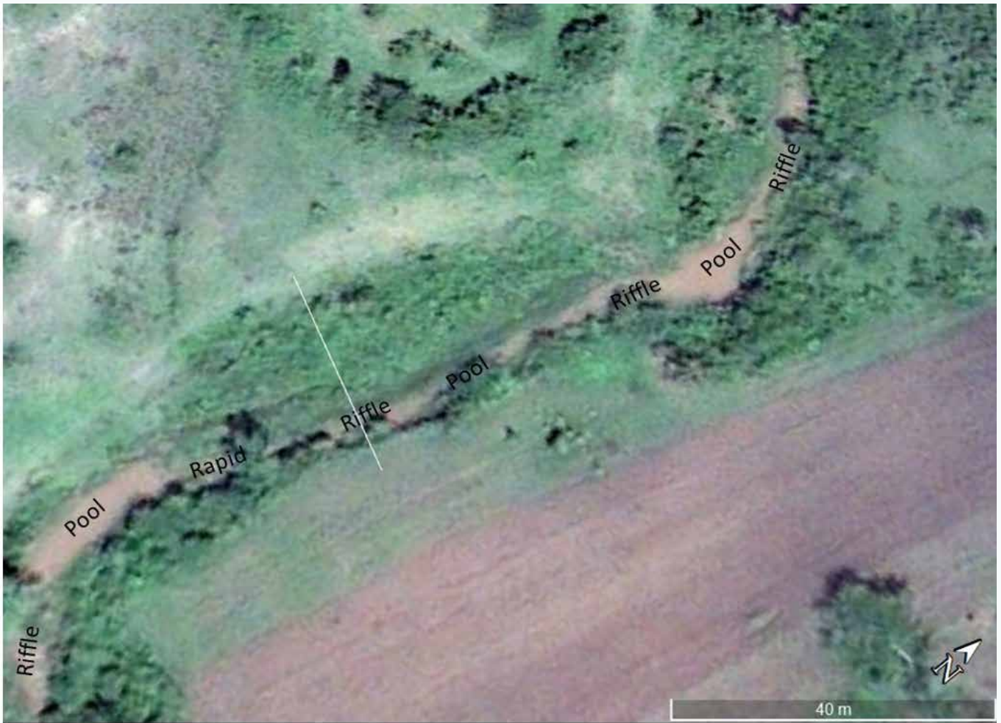
Figure 4 36: A satellite image showing the transect position (white line) and the pool-riffle sequence along the Tigithe River (Google Earth Image date 17 Jan 2010).
