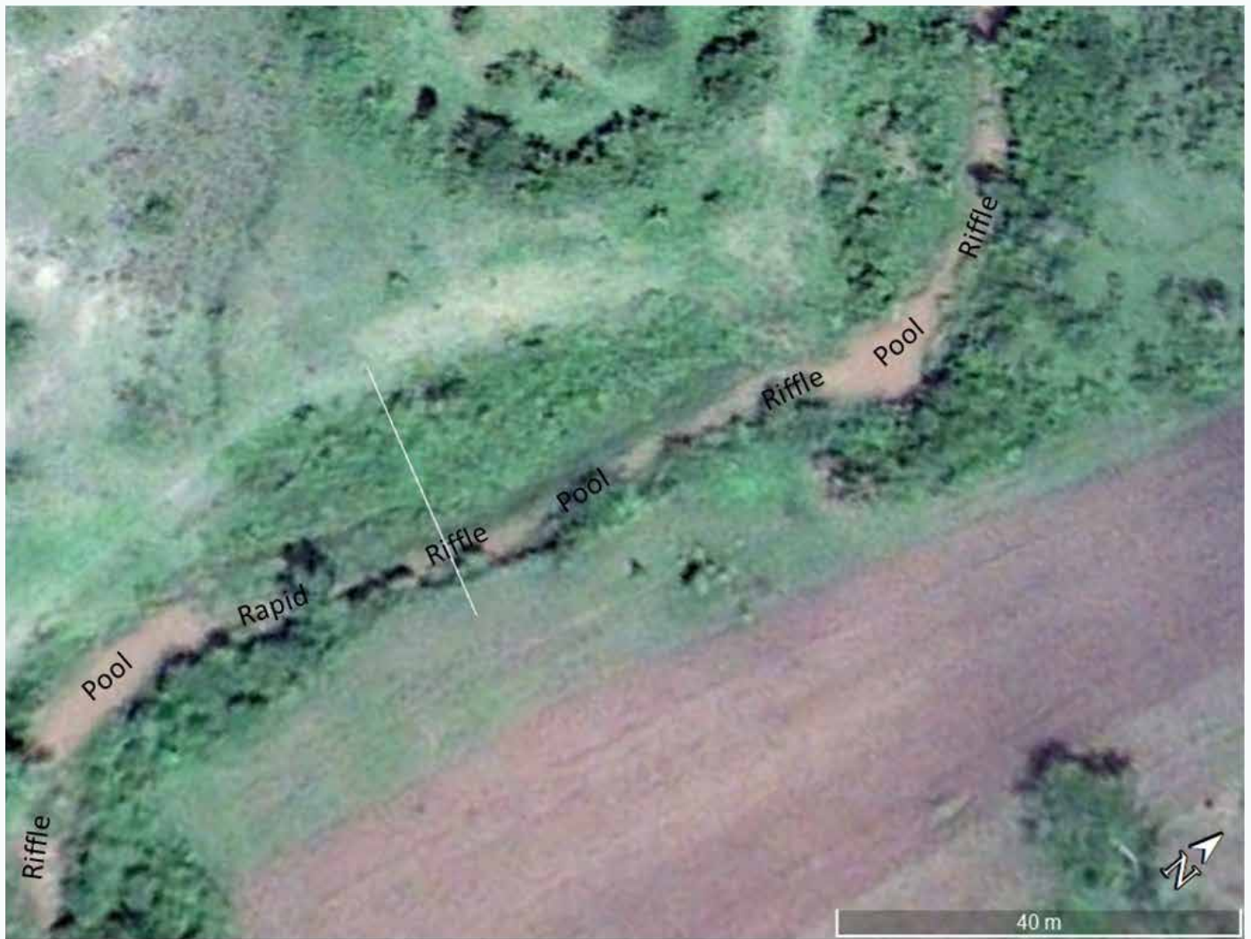
FIGURE 4 36: A SATELLITE IMAGE SHOWING THE TRANSECT POSITION (WHITE LINE) AND THE POOL-RIFFLE SEQUENCE ALONG THE TIGITHE RIVER (GOOGLE EARTH IMAGE DATE 17 JAN 2010).
