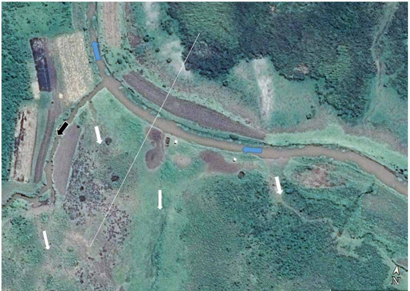
FIGURE 4 58: AERIAL VIEW OF THE MARA RIVER (BLUE ARROWS) AT BISARWI INDICATING THE LOCATION OF THE TRANSECT AND THE BIFURCATION OF THE MARA RIVER UPSTREAM OF THE AVULSION THAT TOOK PLACE IN 1989 (GOOGLE EARTH IMAGE 21 JULY 2017). THE BLACK ARROW INDICATES THE NEW CHANNEL AND THE WHITE ARROWS INDICATE FLOOD CHANNELS.
