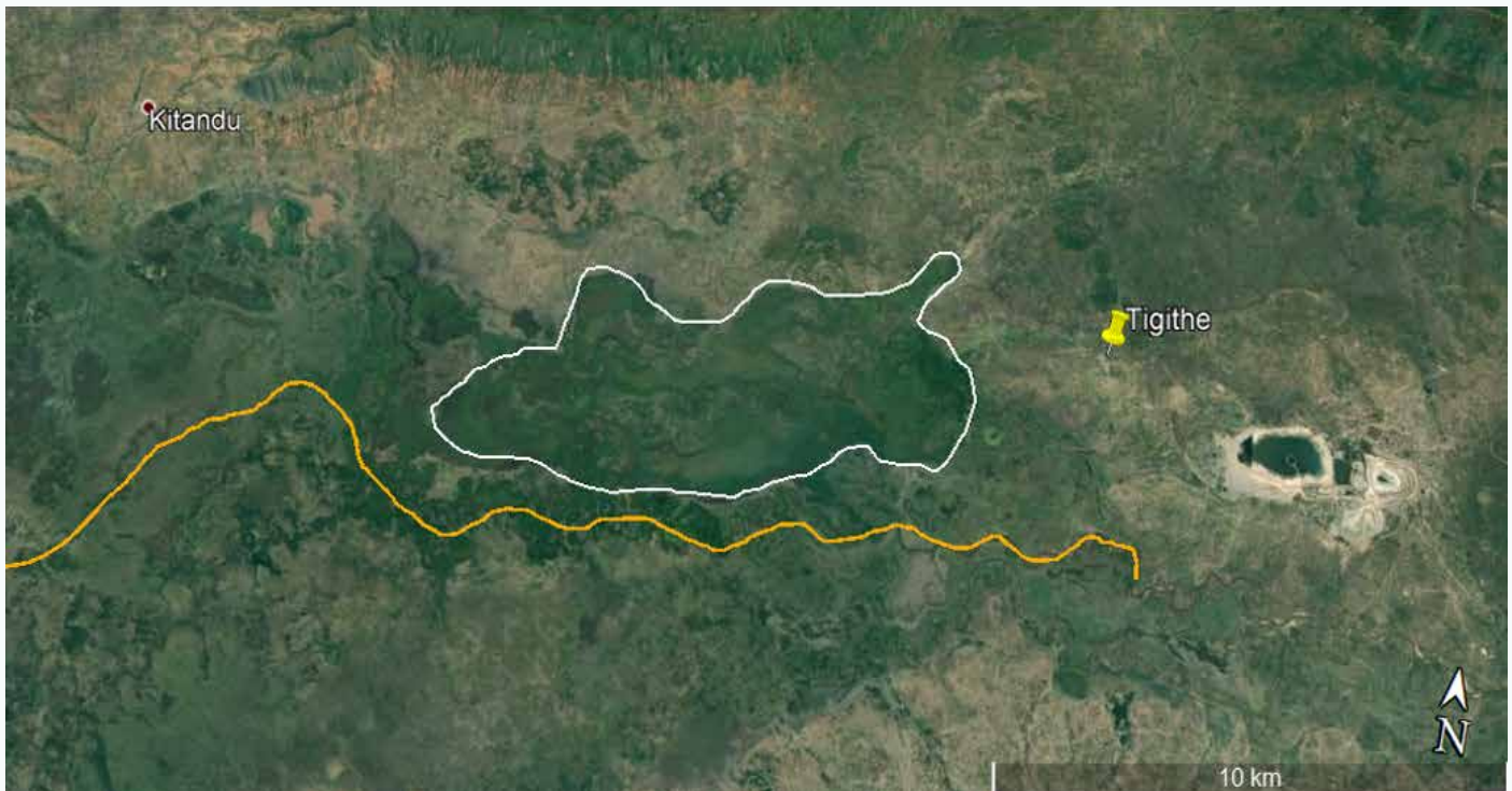
FIGURE 4 38: A GOOGLE EARTH IMAGE SHOWING THE BACK SWAMP (ENCIRCLED BY THE WHITE LINE) FORMED BY THE ALLUVIAL RIDGE/LEVEE (BROWN LINE) ALONG MARA RIVER. THE TIGITHE RIVER DRAINS INTO THE BACK SWAMP PERMANENTLY AND THE MARA RIVER ONLY DURING FLOOD FLOWS. FLOW DIRECTION IS FROM EAST TO WEST.
