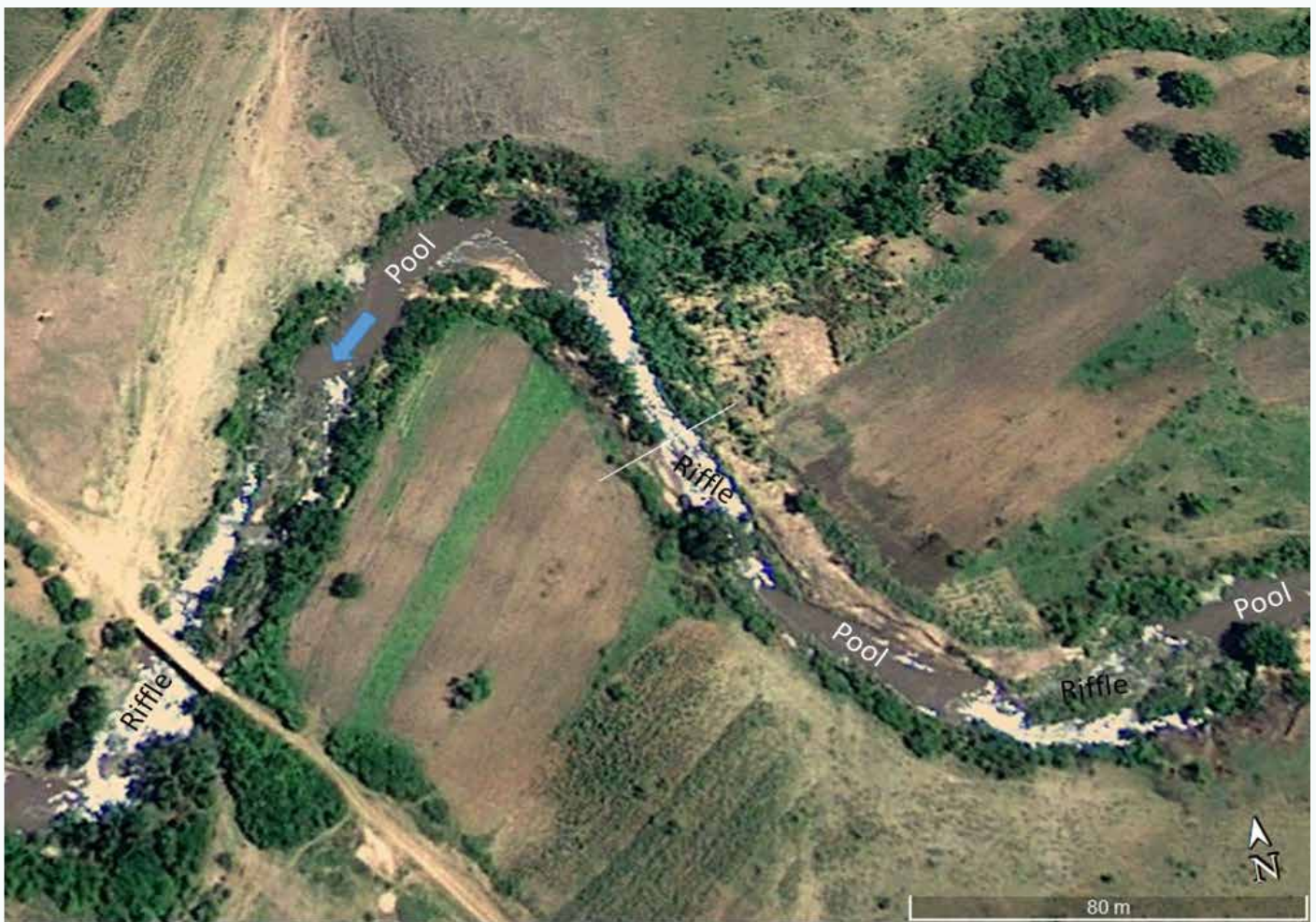
FIGURE 4 16: AERIAL VIEW OF THE TOBORA RIVER SHOWING THE LOCATION OF THE CROSS SECTION, POOLS AND RIFFLES (GOOGLE EARTH IMAGE 24 SEPTEMBER 2010).
