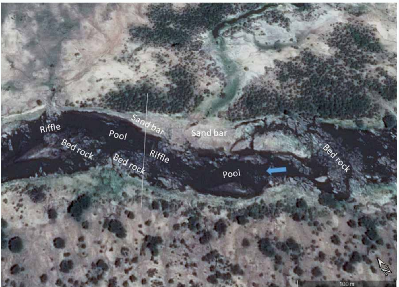
FIGURE 4 6: AERIAL VIEW OF KOGATENDE SITE SHOWING THE LOCATION OF VARIOUS GEOMORPHIC FEATURES AND THE LOCATION OF THE CROSS SECTION.
