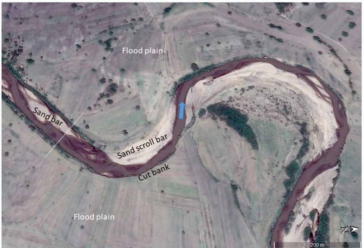
FIGURE 4 47: AERIAL VIEW OF THE MARA RIVER AT MARA MINES SHOWING THE LOCATION OF THE CROSS SECTION, THE MEANDERING PLANFORM AND SANDY BED (GOOGLE EARTH IMAGE DATE 14 APRIL 2017).
