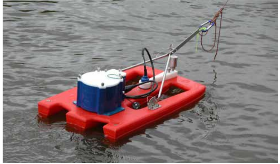
Acoustic Doppler Current Profiler (ADCP)
