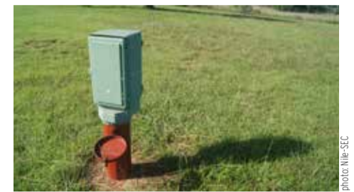
Ground water level monitoring station
