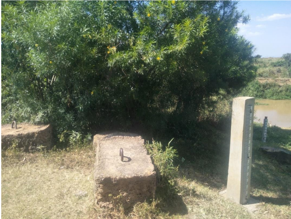
Yala Hydromet Station at Odhuro village. Note that the concrete structure is surrounded by fully grown vegetation on the background
