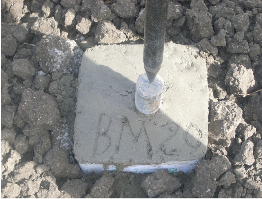
Figure 4.1, a sample of the BMs established in the project area.
