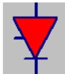
Figure 26: Valve with a standing fault
