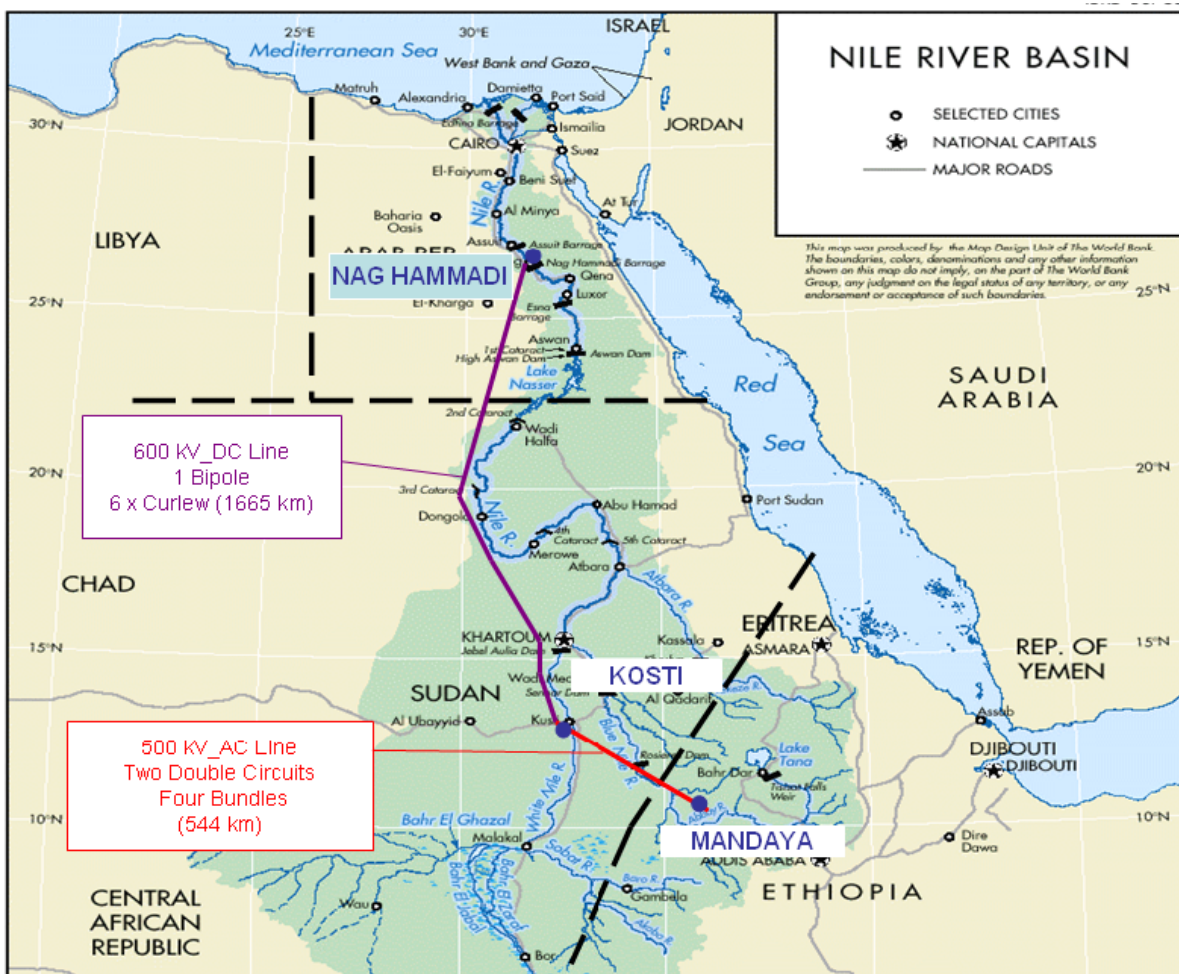
Figure 1 : General View of AC and DC Lines
