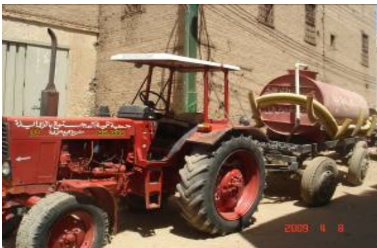
Plate (43): Evacuation Tractor for Waste Water
