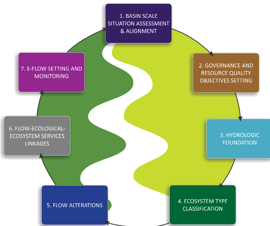
Figure 98: Summary of the seven phases of the Nile E-flows Framework established to direct the management of E-flows in the Nile Basin.
