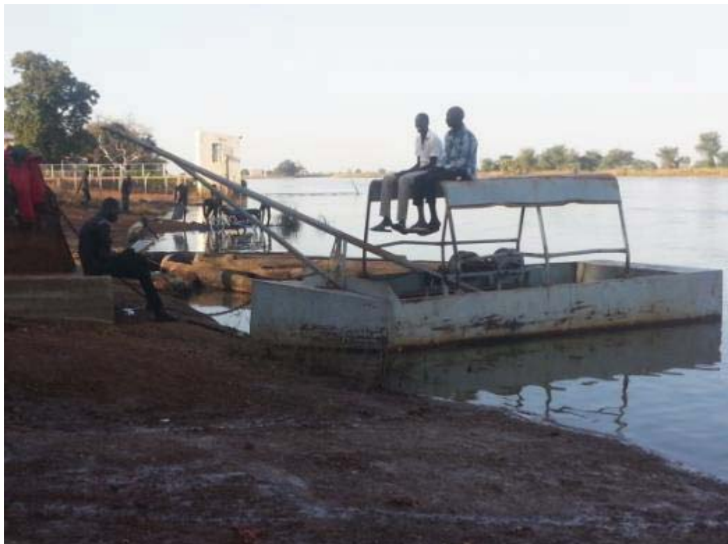
Figure 30: Catamaran used for ADCP discharge measuring downstream of the bridge.
