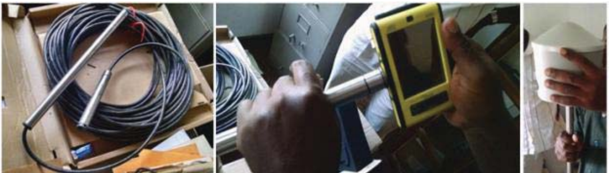
New OTT Orpheus Mini pressure sensor and integrated data logger; downloading data from sensor with PDA; iridium antenna
