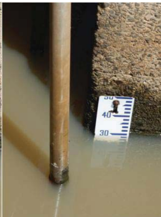
Staff gauge after cleaning algae
