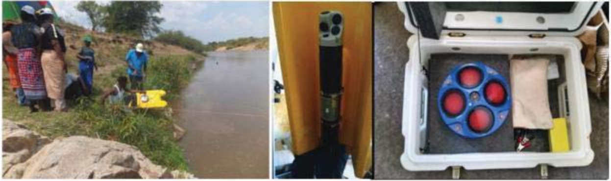
OTT Qliner being used during discharge measurement training; Qliner sensor under boat; backup ADCP
