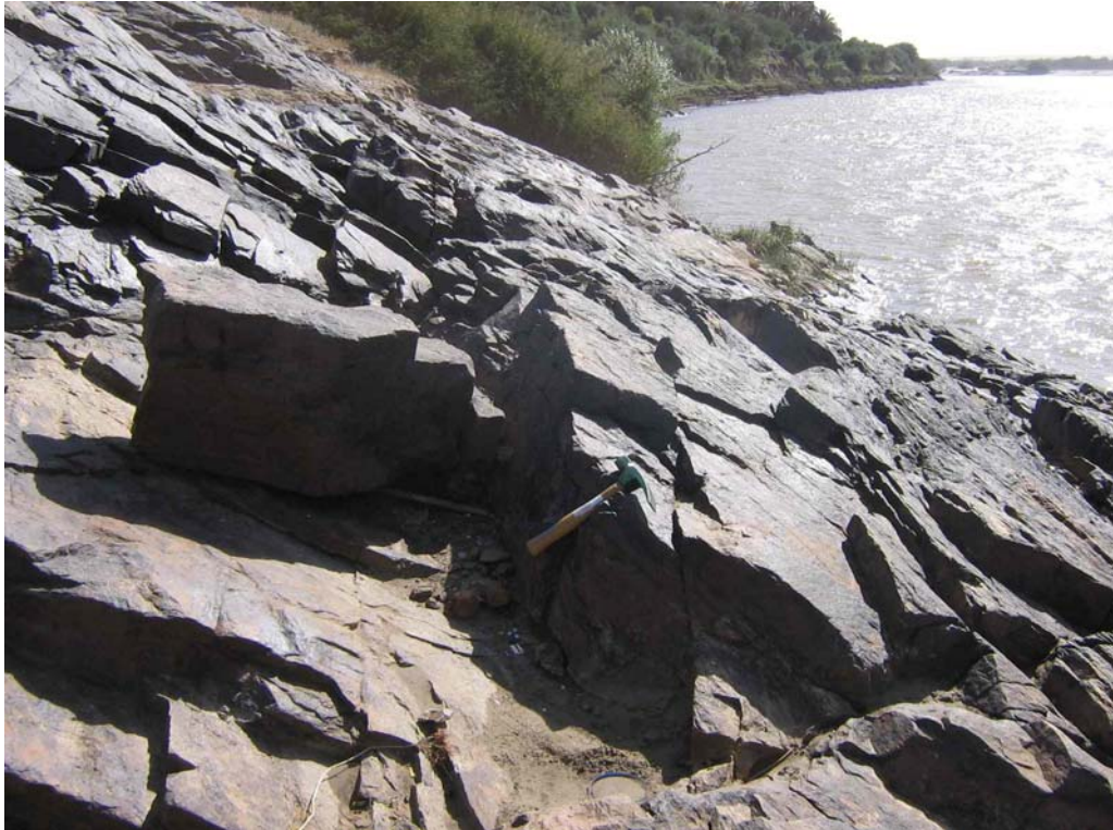
Plate 9 : Meta-sediment and phyllite, quartzite, outcrop at boat crossing, just upstream of bottom of right flank of upstream centreline. Rock type PC4
