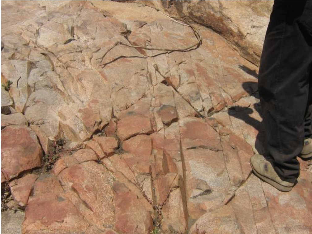
Plate 3: Right bank river section 200m downstream of centre line, gneissic granite intersected by 4 joint sets
