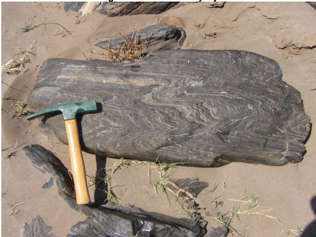
Plate 4: Right bank river section 1000m downstream of centre line, biotite amphibolite gneiss/schist, with isoclinal folds
