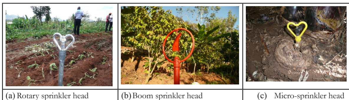
Figure 5.4 Different designs of locally made sprinkler heads (photos by B. Mati)
