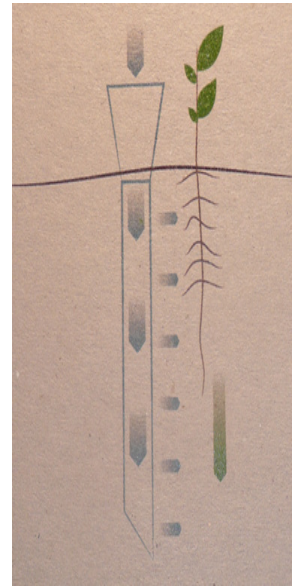
(b) Illustration of Irrigasc deep placement micro irrigation system
