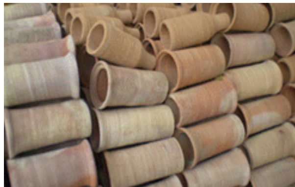
(a) The clay pipes before installation
