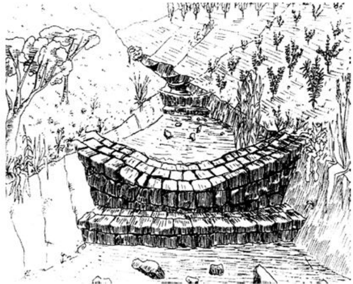
Figure 9: A typical loose stone check-dam
