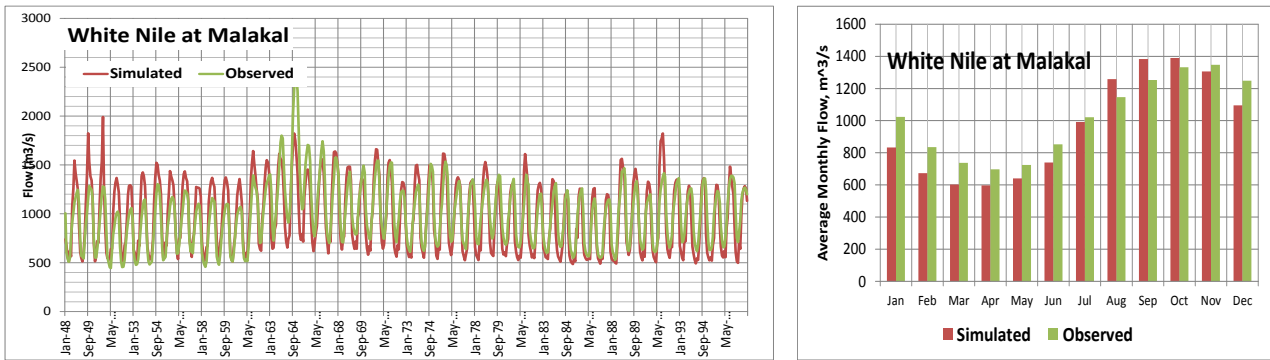
Figure 2b: Observed and (WEAP) simulated monthly flows for White Nile at Malakal
