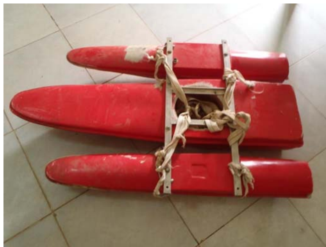
Figure 5 Trimaran type 'boat' for mounting of the ADCP (MoIWR)
