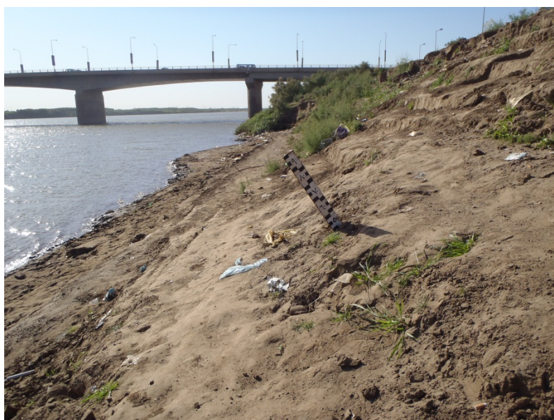
Figure 6 Staff gauge at Khartoum Gauging station at Sobat Bridge (West bank). Oblique gauge and large level gap between gauges
