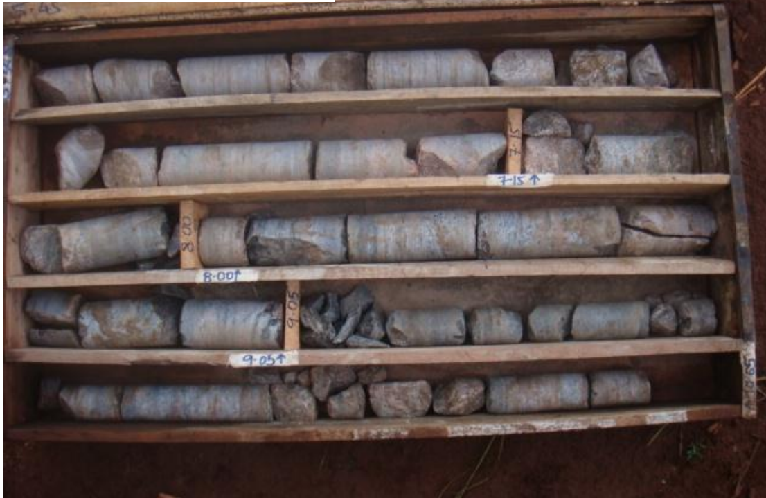
Plate 6.4: Variation of fracturing in both boreholes
