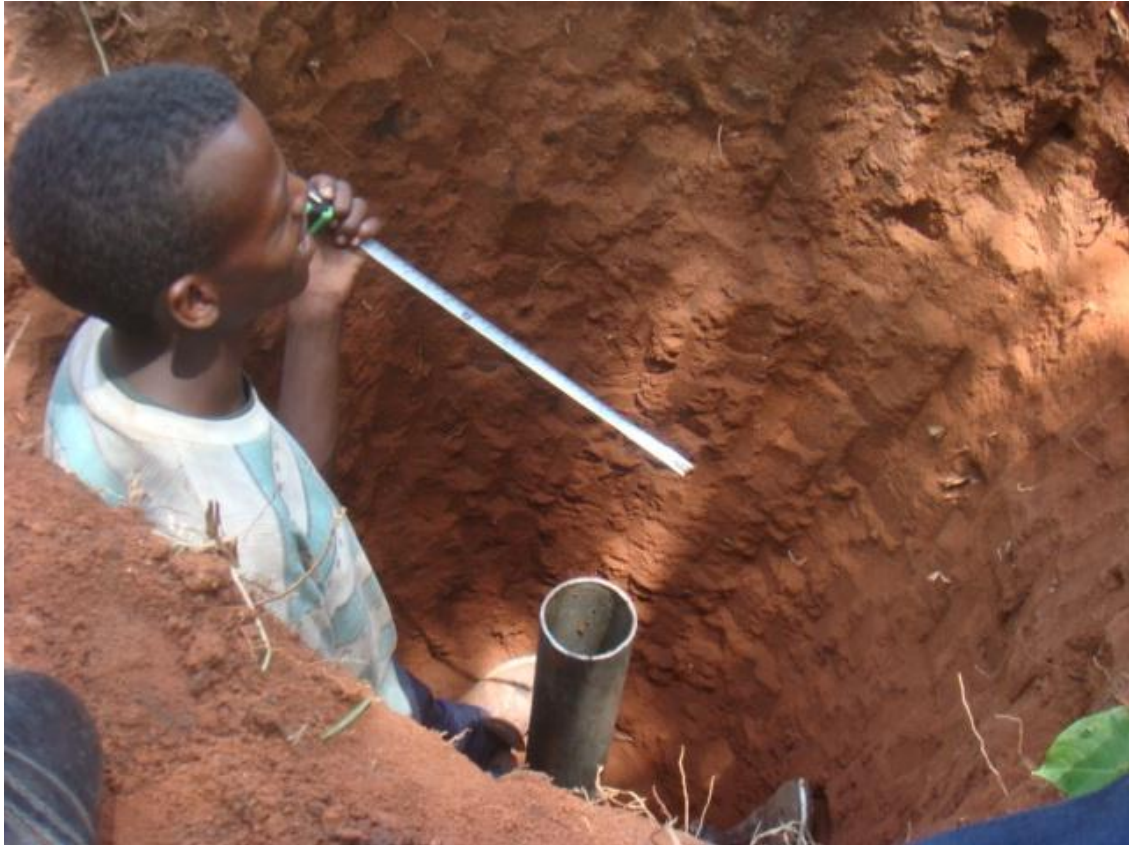
Plate 6.1: Conducting in-situ permeability test at test pit DCTP -23
