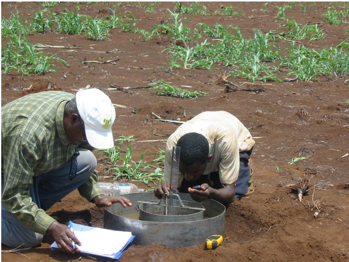
Plate 5.3: Determination of infiltration rates using double ring infiltro-meter
