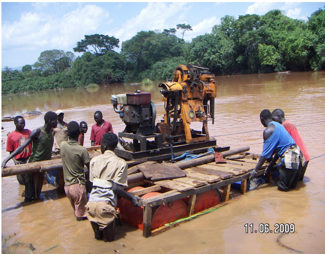
Figure 2. Picture showing a raft carrying drilling rig over Didessa river during inter-borehole movement.
