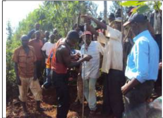
Figure 8: Light Dynamic Cone Penetrometer tests used in Burundi
