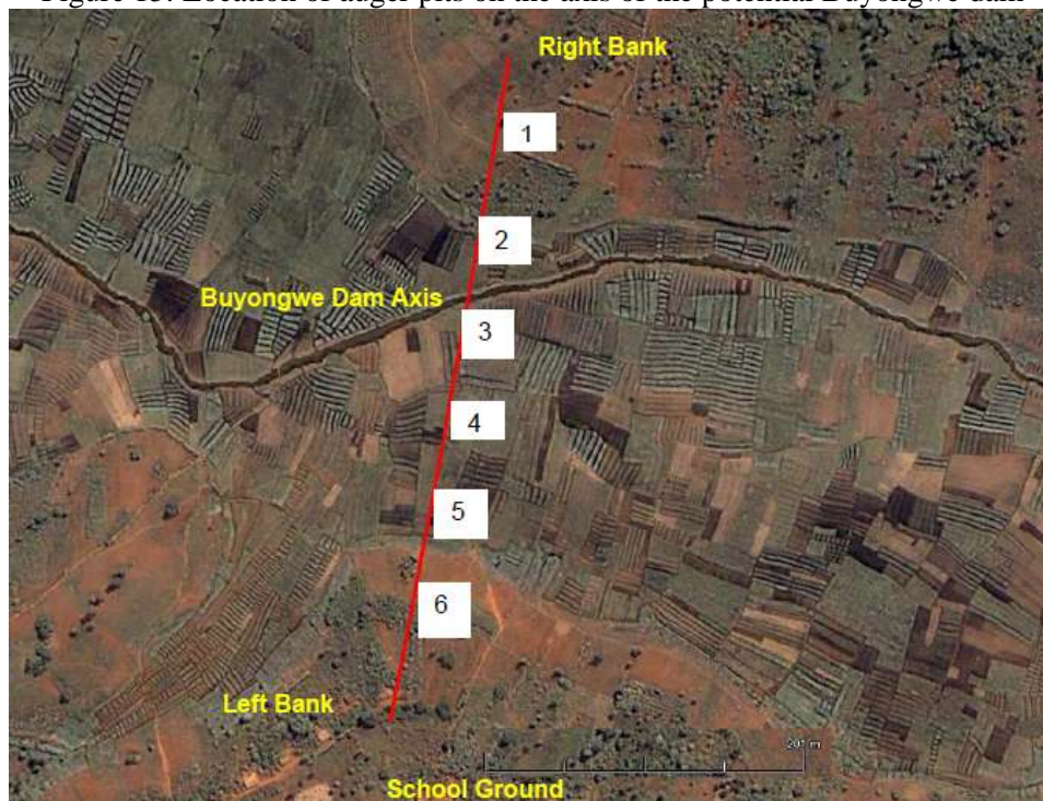
Figure 15: Location of auger pits on the axis of the potential Buyongwe dam
