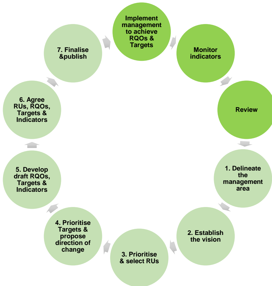
Figure 15: Procedure for the determination of RQOs for the Nile Basin (adapted from DWA, 2011).
