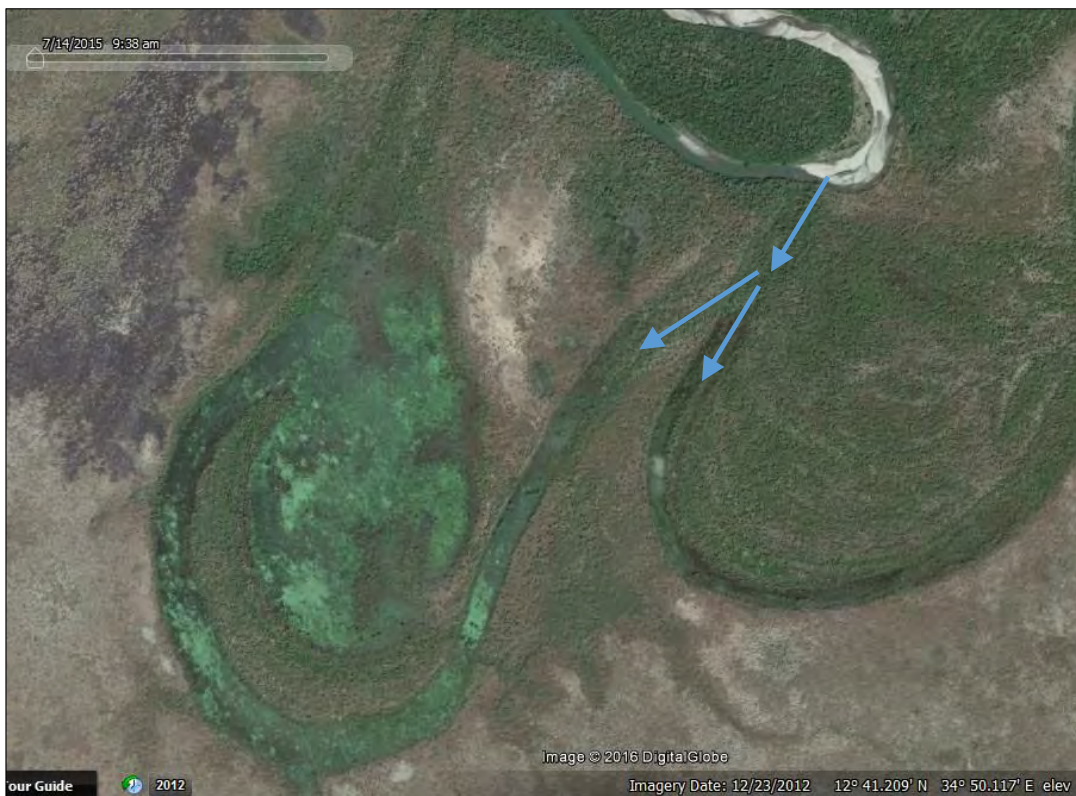
Figure 88: Satellite image (Google Earth ©, date 23 Dec 2012) of portion of the Dinder River and associated Mayas inside the Dinder National Park, showing potential nick point at which the main channel could extensively flood Mayas.
