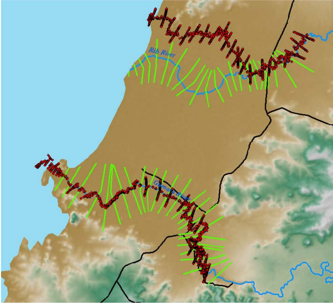
Figure 4-3: Proposed (green lines) and actual survey (red points) for the Gumara and Ribb Rivers.
