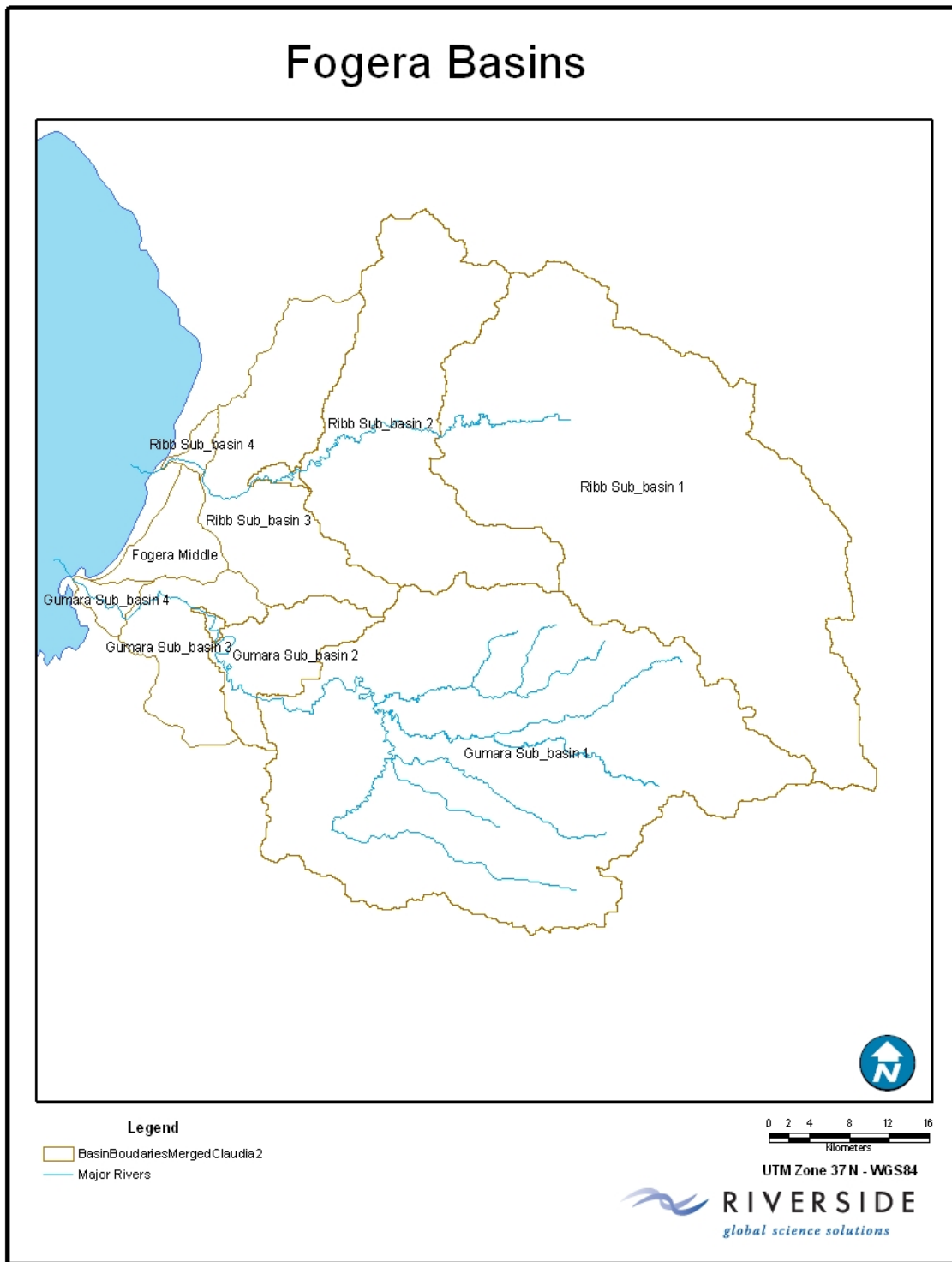
Figure 5-8: Map of the Gumara, Ribb and Fogera middle basins. Fogera middle corresponds to Subbasin 5 of the Ribb River basin schematics in HEC-HMS.
