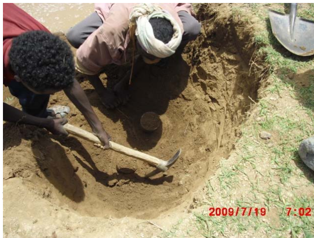
Figure 4-1: Undisturbed Sampling by Core Cutter (Photo Showing during Core Cutter Retrieval: Axum Water Supply Project)
