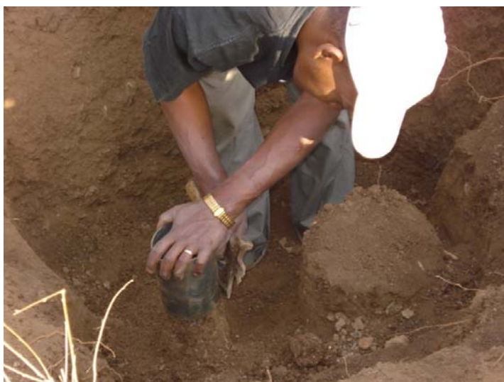
Figure 5-5: Photo Sowing Method of Obtaining a Hand Cut Undisturbed Cylindrical Sampling (Shefe Dam Site, SNNPRS, Ethiopia).
