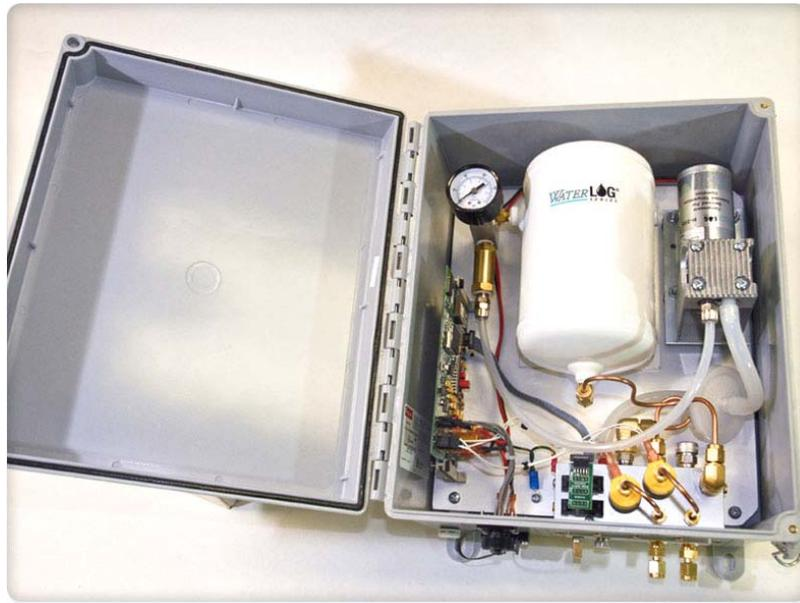
Figure 5-2: single unit bubbler system (WaterLOG YSI incorporated, used by permission)
