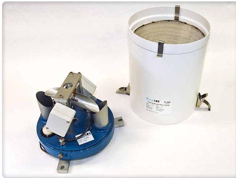
**Figure 5-3: Tipping Bucket (WaterLOG YSI incorporated, used by permission)**
