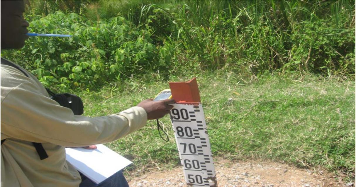
**Figure 16. Testing the accuracy of the GPS in reading elevation**
