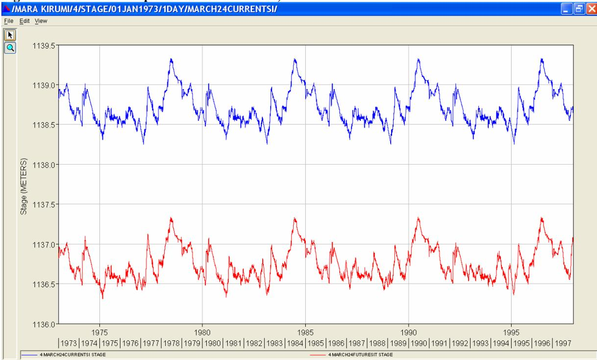
**Figure 60. Water surface profile at cross section 4, current and future situation**
