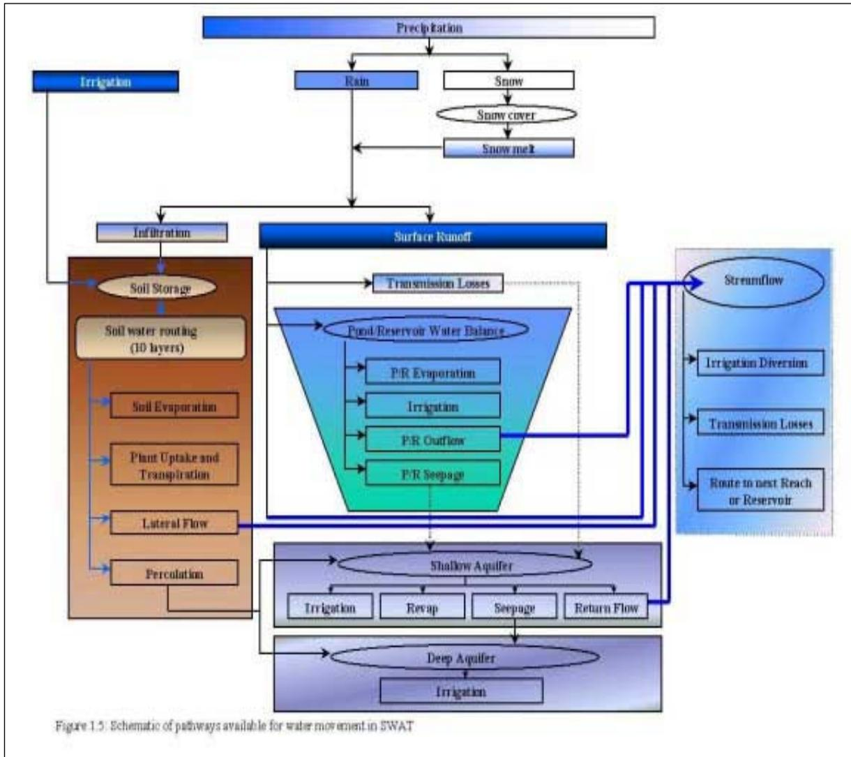
Figure 1.5. Schematic of pathways available for water movement in SWAT
