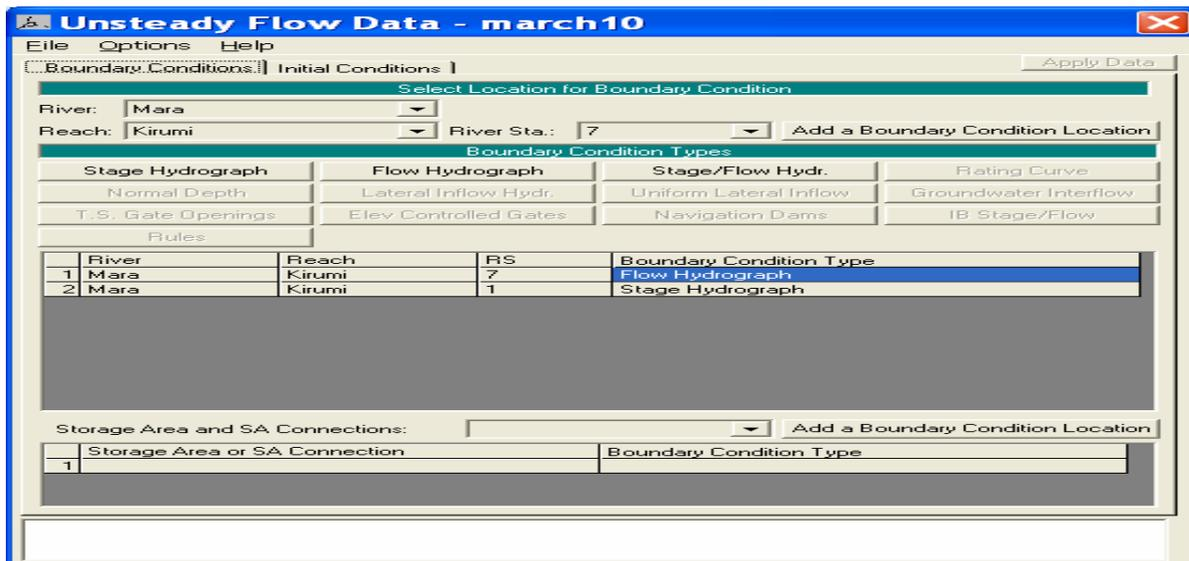
Figure 42. Providing unsteady flow simulation data
