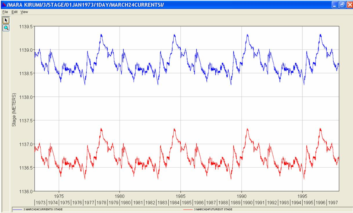
**Figure 59. Water surface profile at cross section 3, current and future situation**
