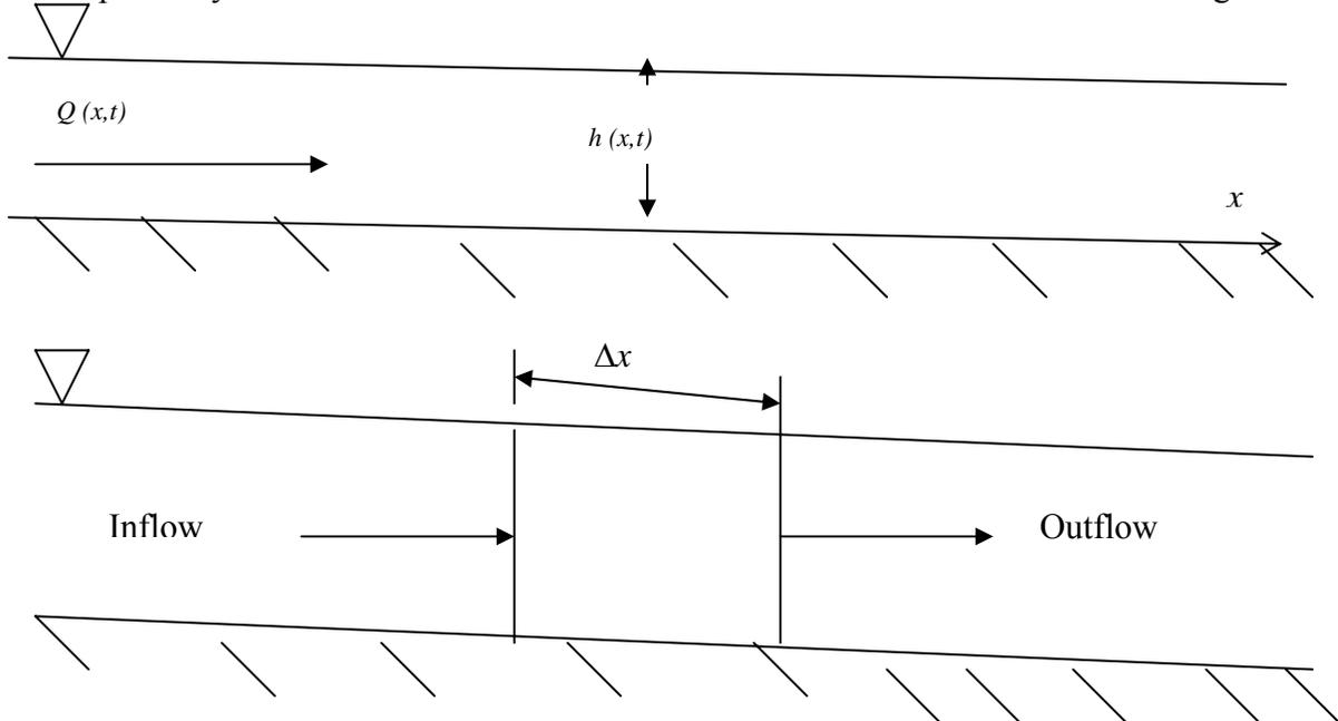
**Figure 11. Control volume for continuity equation**
