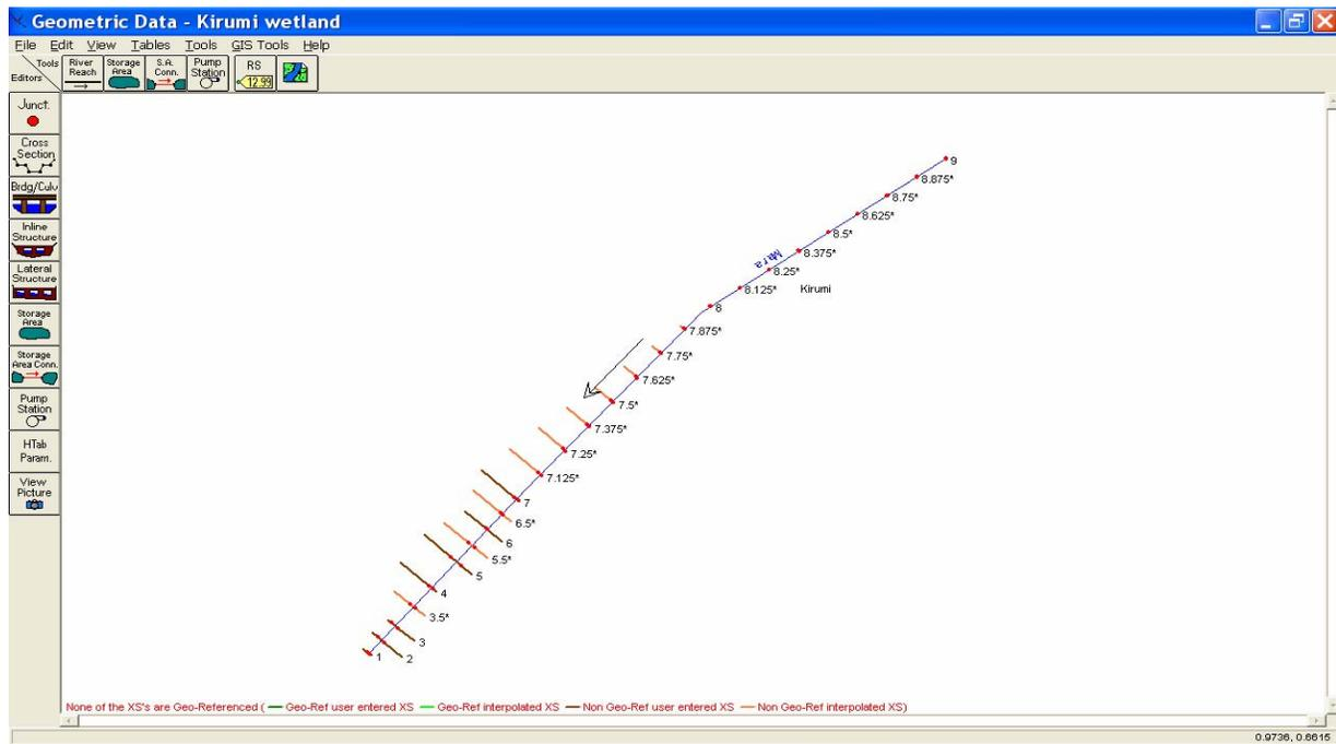
**Figure 49. Revised river schematics with more cross sections**
