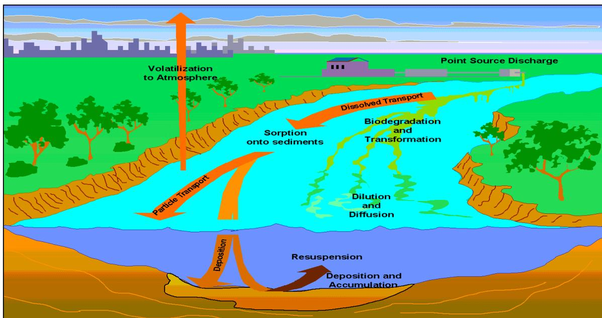
Figure 8. In-stream processes modeled by SWAT.
