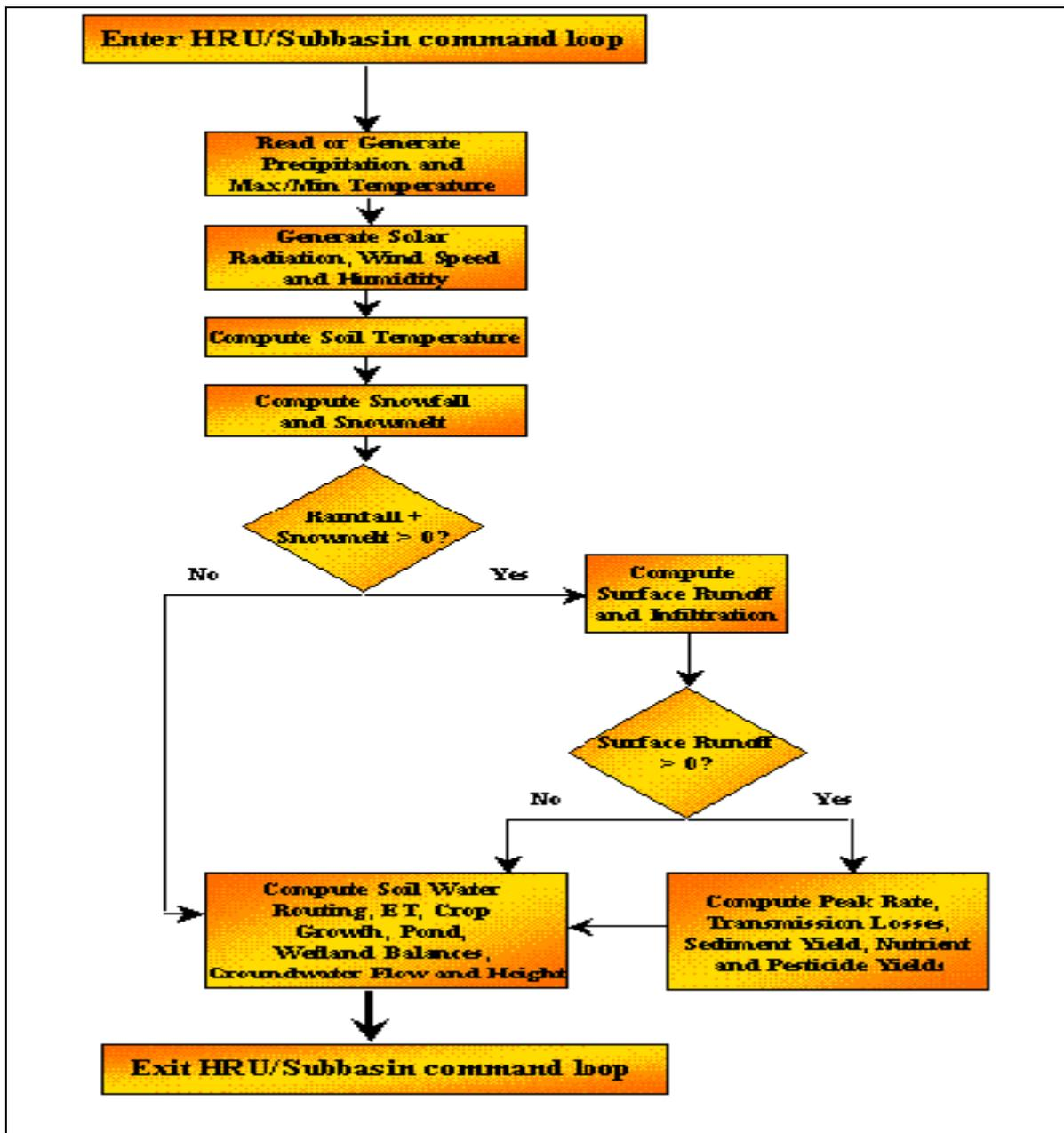
Figure 5. The general sequence of processes used by SWAT to model the land phase of the hydrologic cycle. Source (Neitsch *et al.*, 2002).
