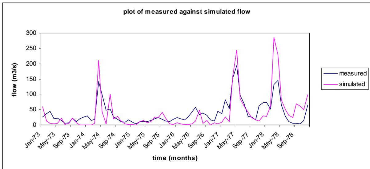
**Figure 39. Fitting the measured against the simulated flow**
