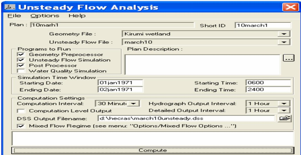
Figure 45. Setting up a trial unsteady flow simulation
