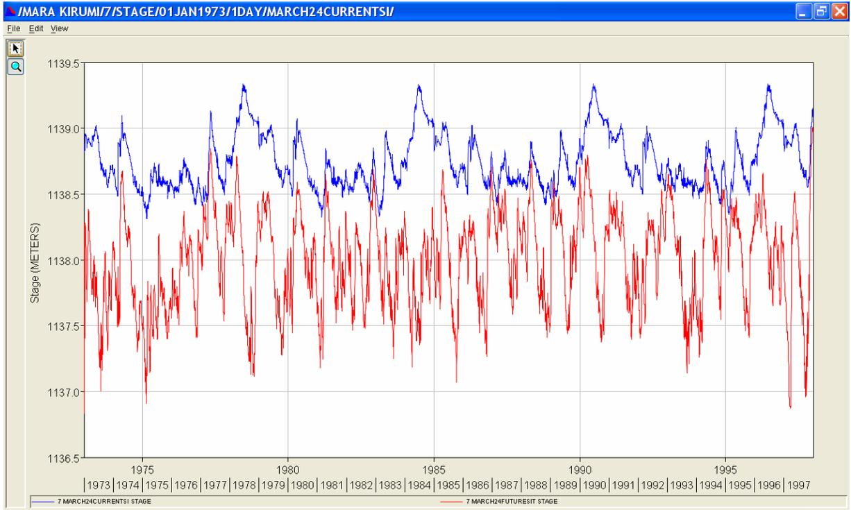
Figure 63. Water surface profile at cross section 7, current and future situation
