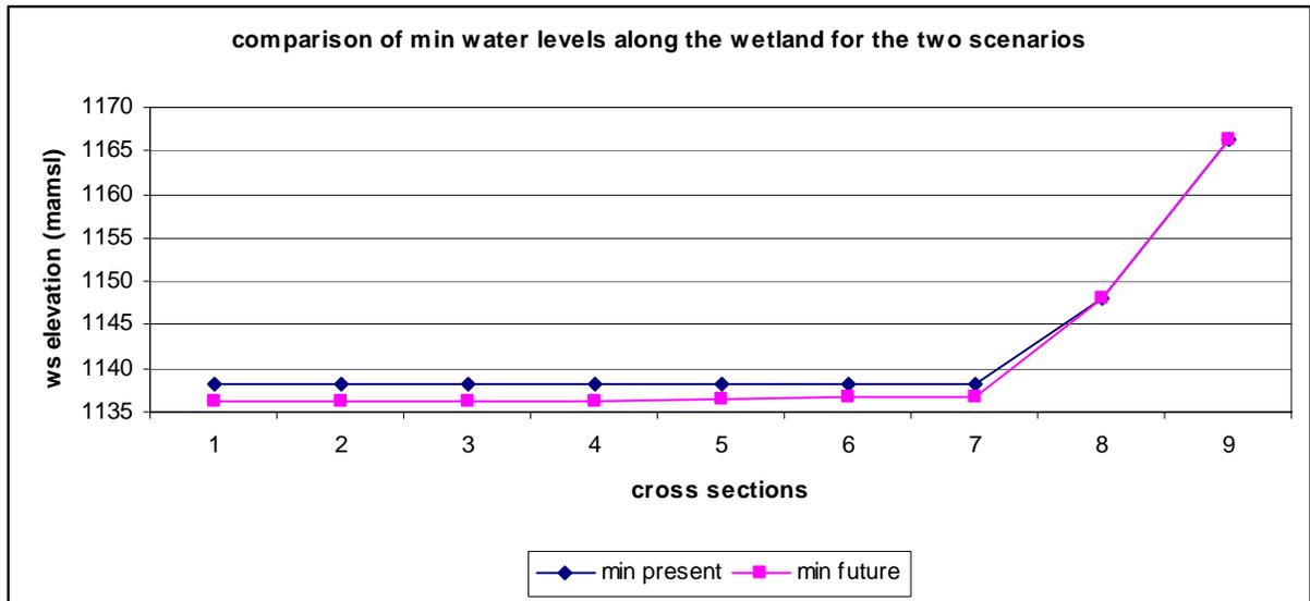
Figure 79. Comparison of minimum water levels along the wetland for the two scenario
