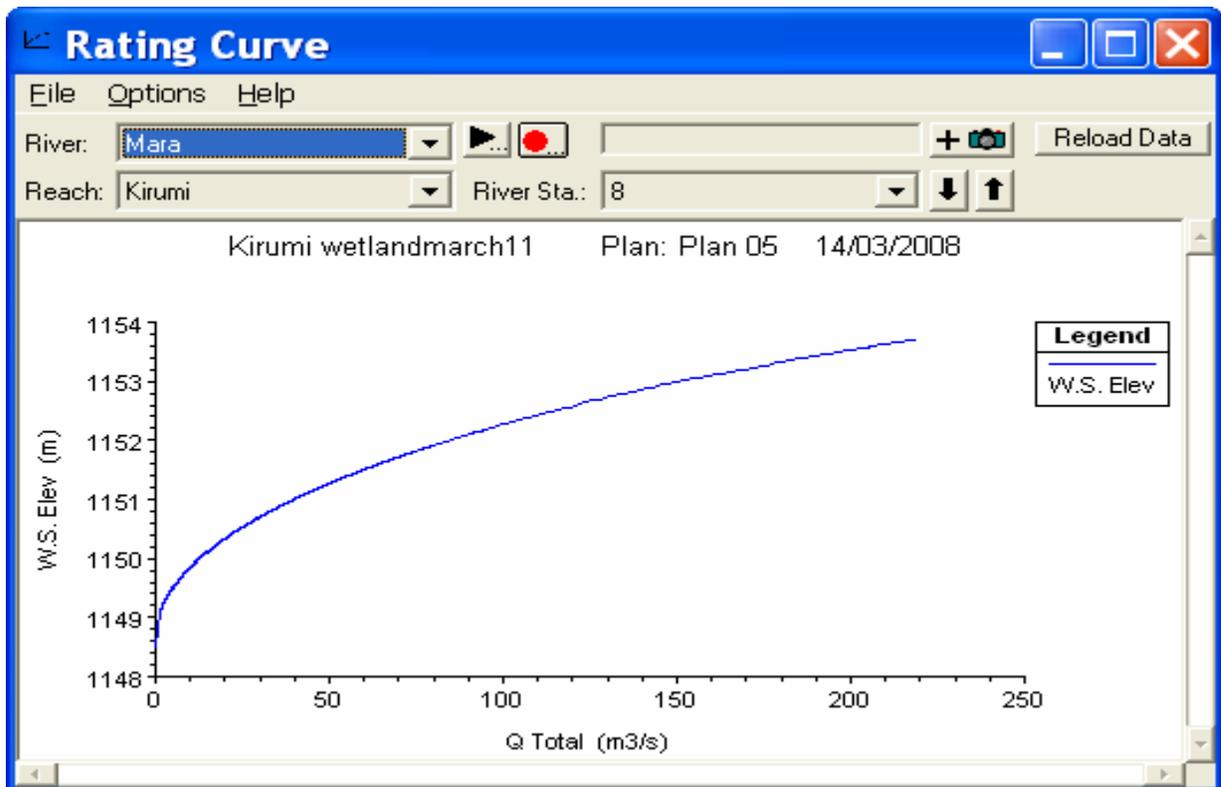
Figure 52. Rating curve at new cross section 8
