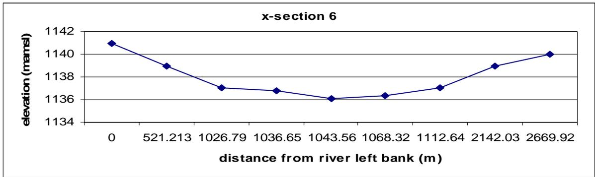
Figure 22. Profile at cross section 6
