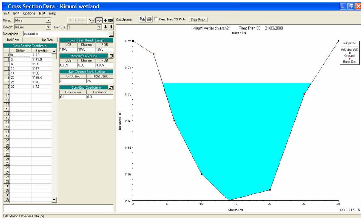
Figure 54. Water surface profile at cross section 9 with an increased n value
