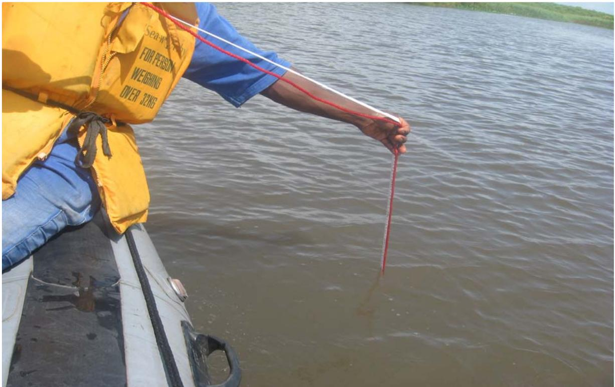
Figure 13. Making soundings of the river cross section
