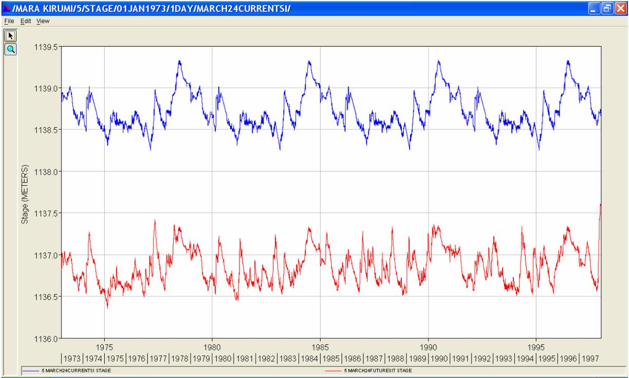
**Figure 61. Water surface profile at cross section 5, current and future situation**
