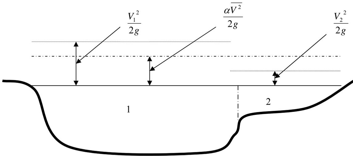
**Figure 10. Calculation of mean energy in the cross section**
