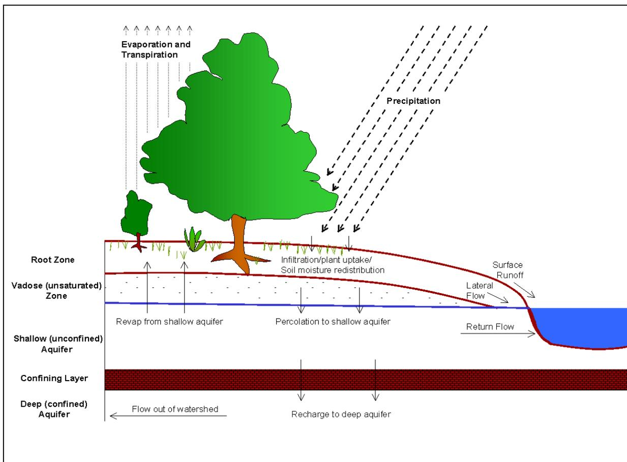
Figure 6. Schematic representation of the hydrologic cycle. source:(Neitsch *et al.*, 2002).
