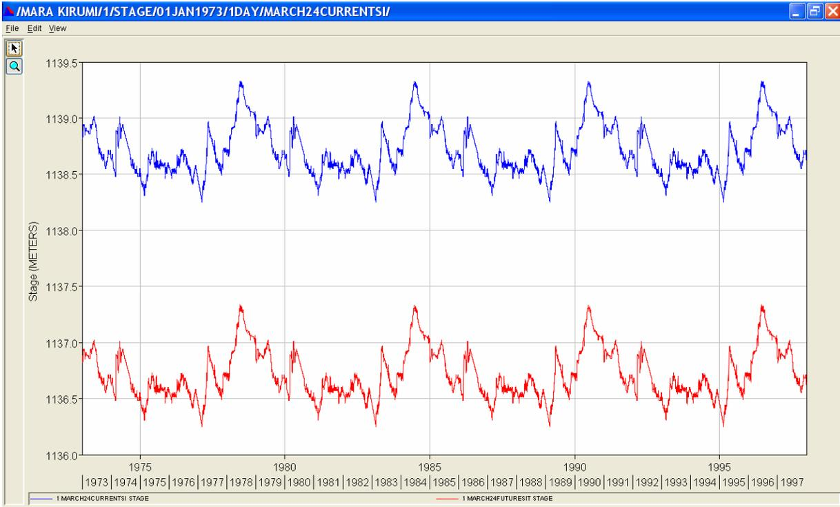
**Figure 57. Water surface profile at cross section1, current and future situation**
