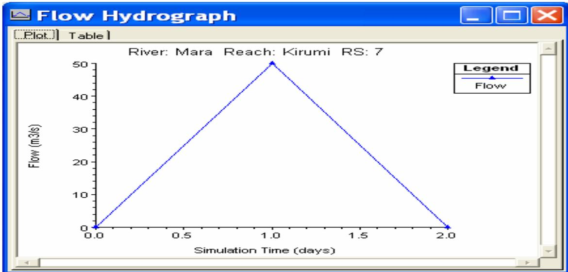
Figure 43. Trial upstream boundary condition
