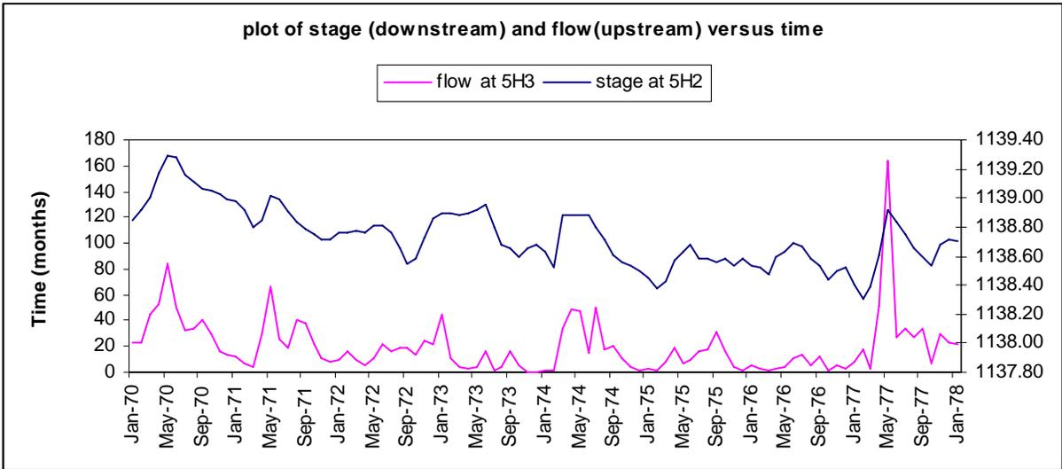
Figure 27. Correlation between measured flow and lake water level
