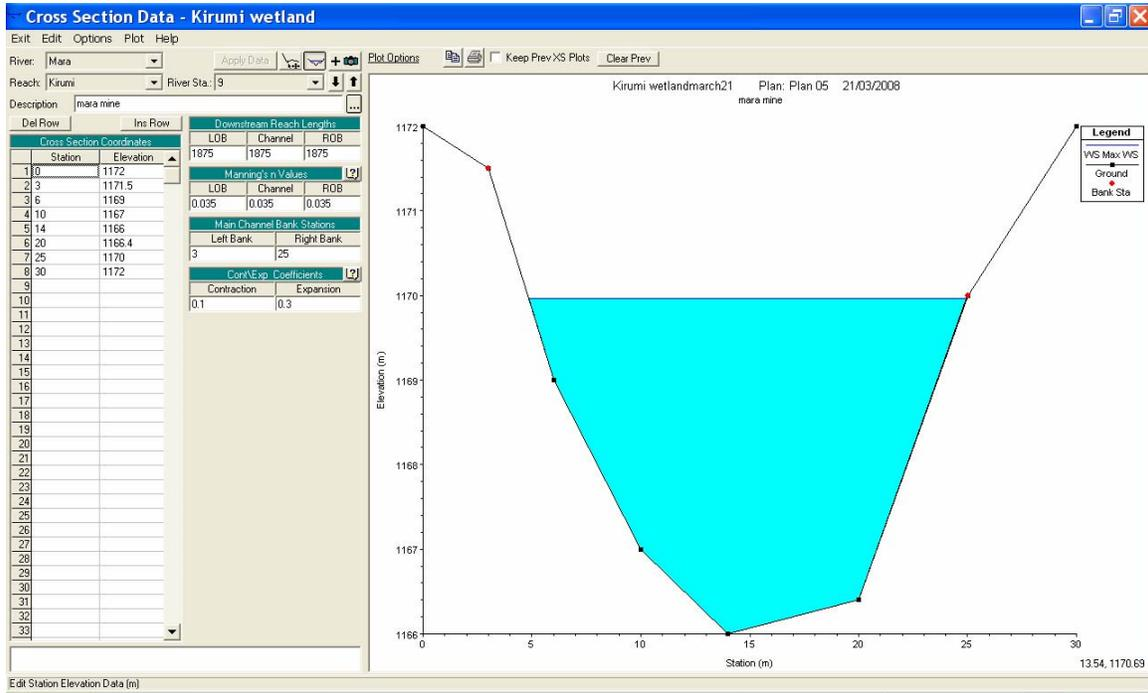
Figure 53. Water surface profile at cross section 9
