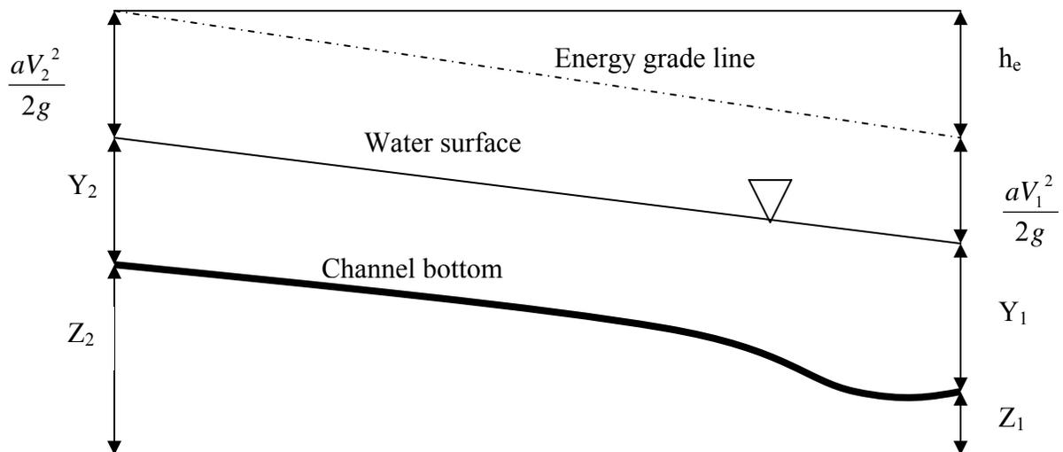
Figure 9. Terms of energy equation used in HEC RAS model.
