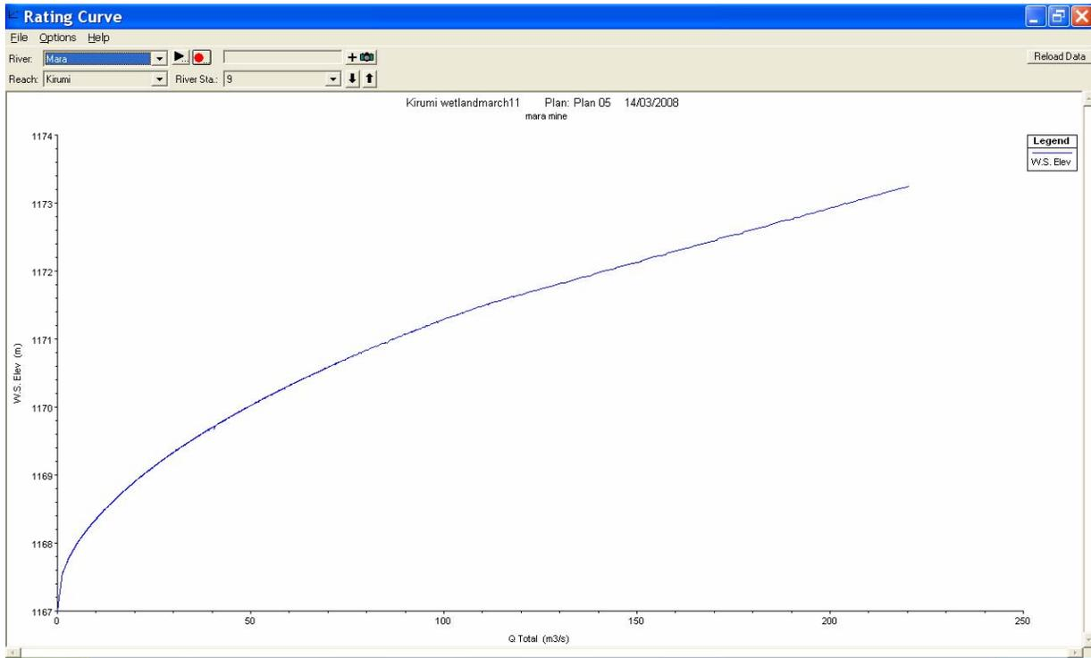
Figure 51. Rating curve at new cross section 9
